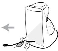
To increase the length of the power cord: Grasp the power cord (not the power plug) and gently lift it out of the slot, then feed it into the coffeemaker. Lock the cord in the slot when finished.
